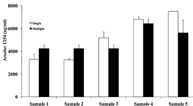
**Figure 3.** Aroclor 1254 content in aroclor soil/sediment samples: comparison of values obtained in single- and multianalyte aroclor 1254 ELISA formats. Each bar represents the mean  $\pm$  SEM (standard error mean) of three or four measurements. Statistical analysis compared values obtained in the single vs multiple assay formats for each sample independently. Values of all tested samples did not differ significantly at  $p < 0.05$ .
