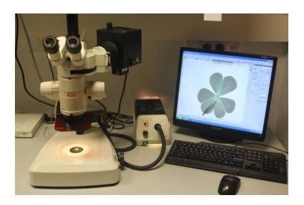
Leica MZFLIII stereomicroscope (Germany) with Nikon DS-Fi1 digital camera and NIS-Elements software(Japan) for bright field and fluorescence imaging.
