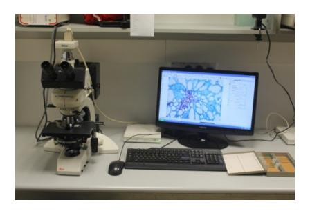
Leica DMLB epi-fluorescence microscope( Germany) with DS-Fi1 digital camera and NIS-Elements BR3.0 software(Nikon).
